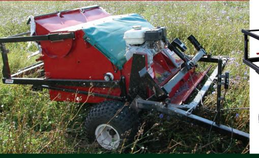
The drawbar has 3 ▶ operating positions seen here with maximum offset to allow collection from untracked foliage.
