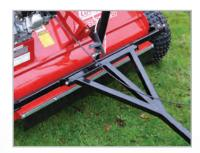
This model has a simplified drawbar and is towed in the central position.
