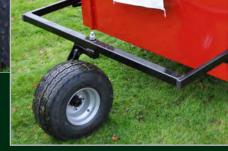
Flotation wheels, including this rear castor wheel, are fitted as standard to ensure easy towing by any suitable vehicle over soft or rough ground conditions.
